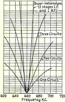
In the diagram it is assumed the receiver in each case is tuned to a frequency of 660 kilocycles (455 meters). The signal field strength required to produce a standard signal of comfortable
