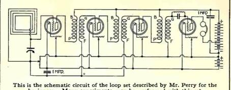
This is the schematic circuit of the loop set described by Mr. Perry for the beginners. Many experiments may be performed with this set which will lead to an increased interest in radio
