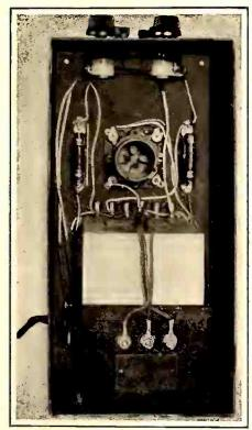
In this photograph is shown the 171 power compact whi.h furnishes A current for the 171 tube filament; B and C voltages for the 171 power tube, and the B voltages for the balance of the receiver
